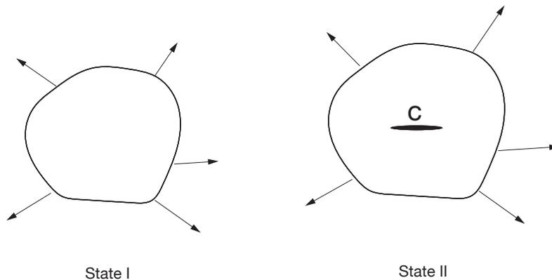
In general it is difficult to calculate the change in the potential energy. For example consider the two states shown above; it is almost impossible to ask for the change in the potential energy with and without the crack.
